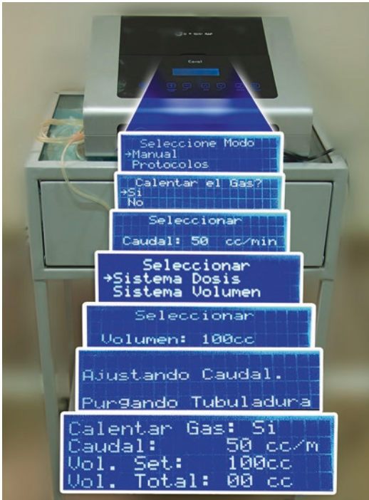
Fig. 11.6 Treatment settings. (1) Select mode (preset settings or manual settings). (2) Warm gas: always. (3) Set flow. (4) Select dosage system. (5) Set volume to be injected. (6) Always purge tube system. (7) Device is ready to do treatment
